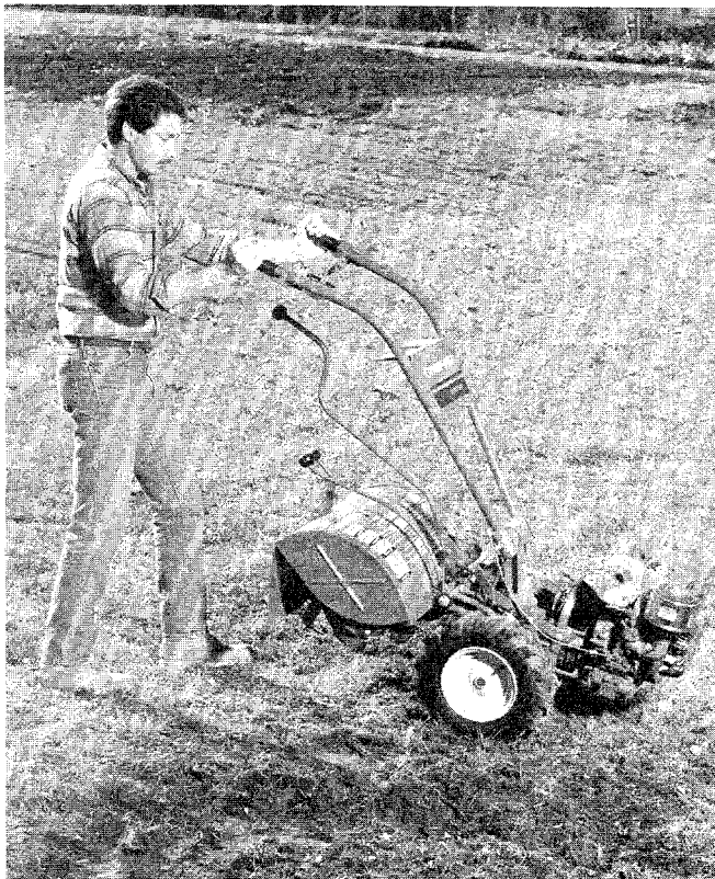
3-9: Lift the handlebars and find balance point. Then PUSH handlebars to swing tiller around.
